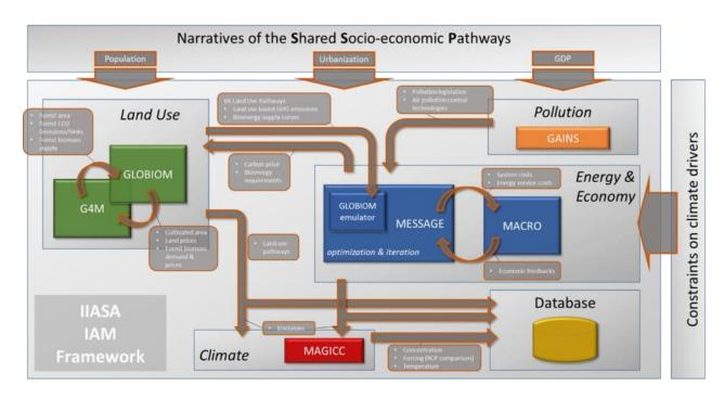
Figure 52. Overview of the IIASA IAM Framework. Coloured boxes represent respective specialized disciplinary models which are integrated for generating internally consistent scenarios. Figure from Riahi et al. (2016).
