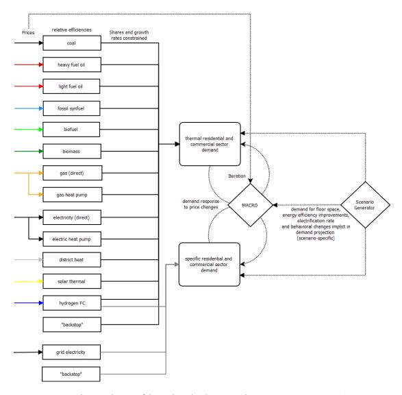
$\textit{Figure 57}. Schematic \textit{ diagram of the residential and commercial sector representation in \textit{MESSAGE} ix} \\$
